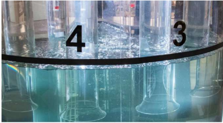
This 2½-meter tall plexiglass model is a true copy of the planned pumping station by Kalvebod Brygge in Copenhagen. The purpose of the model is to test that the pumps will work as intended, when the pumping station is constructed in its full size.
