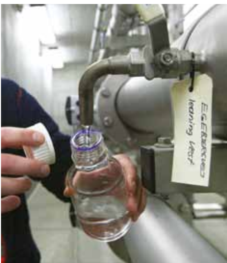
Taking a water sample to be sent to the laboratory for analysis.
